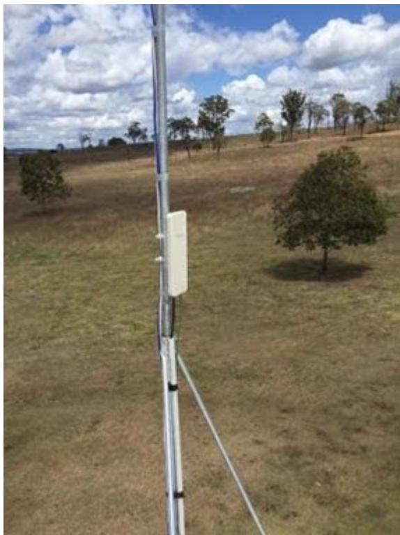
Point to Point connection antenna on a pole mount holding a Fixed Wireless antenna.
