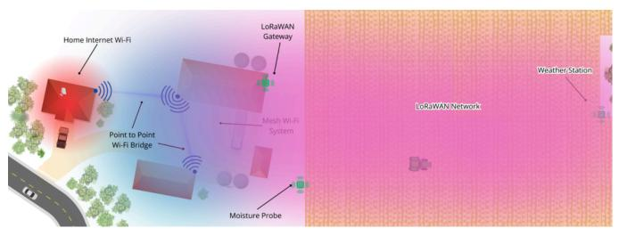
Above is an example of LoRaWAN network spreading coverage further across a farm.
