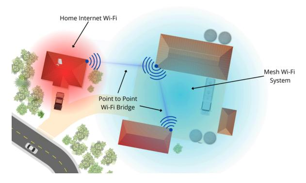
Above is an example of Wi-Fi bridges and Mesh systems spreading coverage across a farm.
