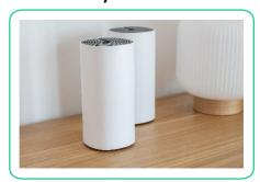
A Wi-Fi mesh system uses multiple devices (called nodes) placed around your home to create a single, seamless network.
