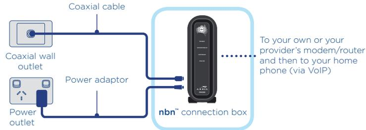
**Note:** Setup may vary slightly from what is shown here for installations with a pay TV service. Visit [nbn.com.au/HFC](http://nbn.com.au/HFC) to find out more.
